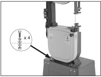
Figure 13. Bandsaw assembly attached to the stand.
